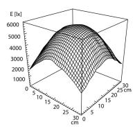
light source LED work equipment electronic plug-in ballast 100-240 V, 50/60 Hz connected load power consumption env. 13 W luminous flux approx. 750 lm light distribution direct direct ratio approx. 100 % colour temperature neutral white colour temperatur approx. 4.000 K
