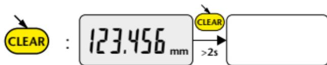
In stand-by mode, the value of the origin is retained by the sensor (SIS mode), and the instrument automatically restarts with any movement of the measurement probe, RS command, *Bluetooth*<sup>®</sup> request or press of a button.
