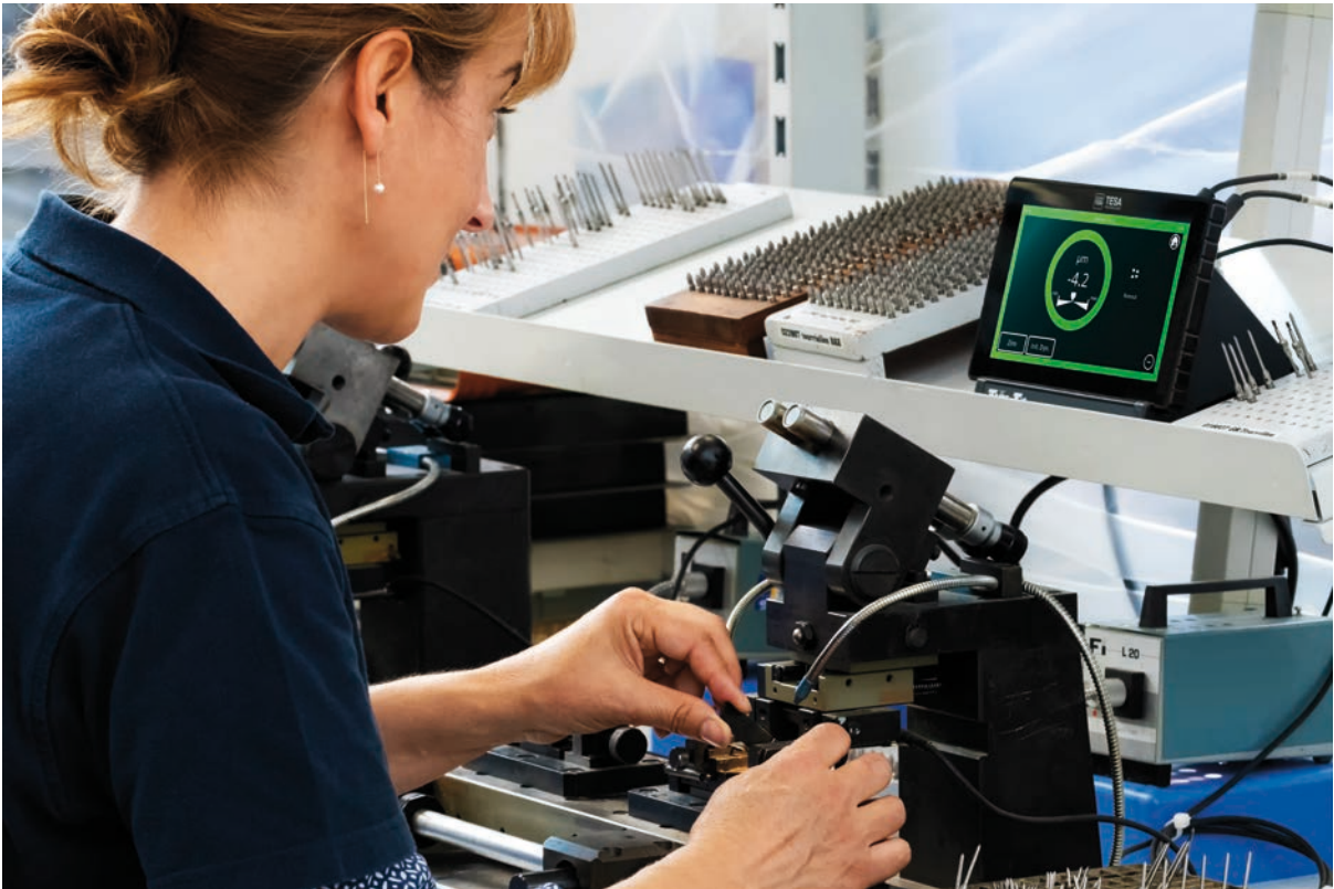
Concentricity measurement before assembly of cylindrical parts
