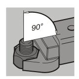
Pull steadily and without any interruption, particularly during the final phase, until you feel a jerk and hear a click. The torque level set on the scale has now been reached.
