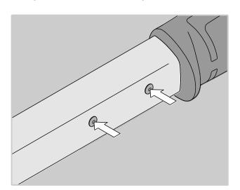
The screw which is closest to the end of the handle is primarily for adjusting the lower end of the scale range.
