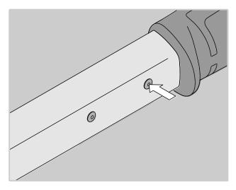
The screw which is closest to the head is primarily for adjusting the upper end of the scale range.
