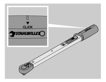
Controlled counter clockwise tightening is possible by turning the MANOSKOP® over. Exceptions: The MANOSKOP® 721/5, 721/15 and 721/20 Quick cannot be used for counter clockwise tightening. Counterclockwise tightening is possible with the MANOSKOP®721/30 Quick by means of a square drive which is pushed through.
