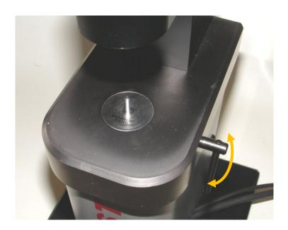
To release the counter-tip, remove the mirror and turn the lever.
