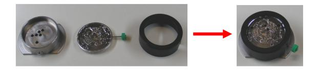
3. Place the movement on the Ebatest. The mirror allows to easily set the correct fitting hole on the pin (each hole corresponds to a wheel position on the movement and is specific to this movement).
