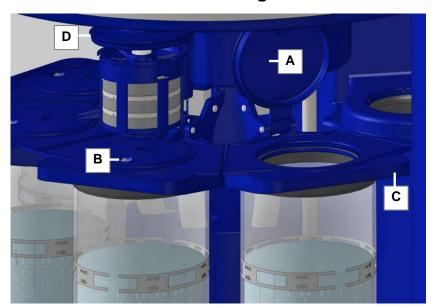
Fig. 3.8. Media tank cover and folding cover
