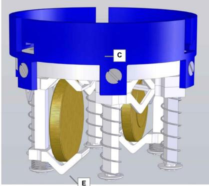
Fig. 6.2.2. Movement hold with clamped parts (simplified display).
