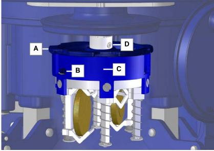
Fig. 6.3.1. Movement holder attached
