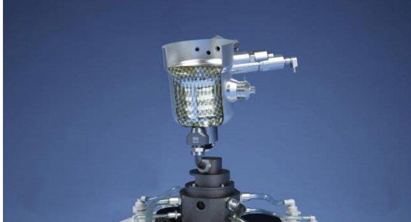
Fig. 3.1.2 View of cleaning basket in cleaning chamber
