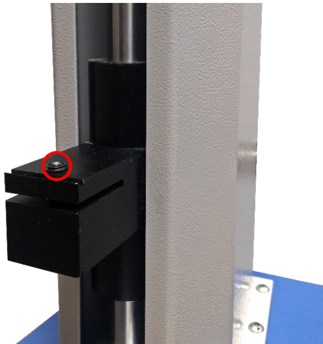
▲MultiTest- dV Dovetail, note the grub screw circled in red
