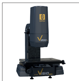
Visio 200 V3 Mot. Measuring range 200x100x150 mm
