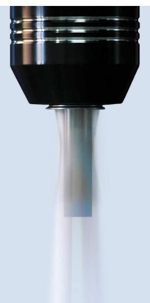
Optimized coolant emission: GZB-S 20/16 for peripheral cooling in a TENDO E compact.
